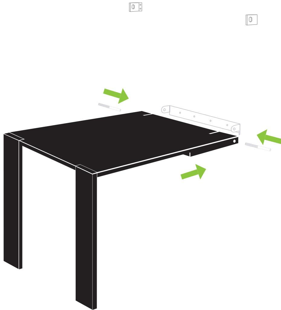
Fix the table legs, lift the table up and slide the grooves on the table surface into the **Lower Wall Mount** on the wall. Screw in the bolts with an Allen key on both sides of the table.
