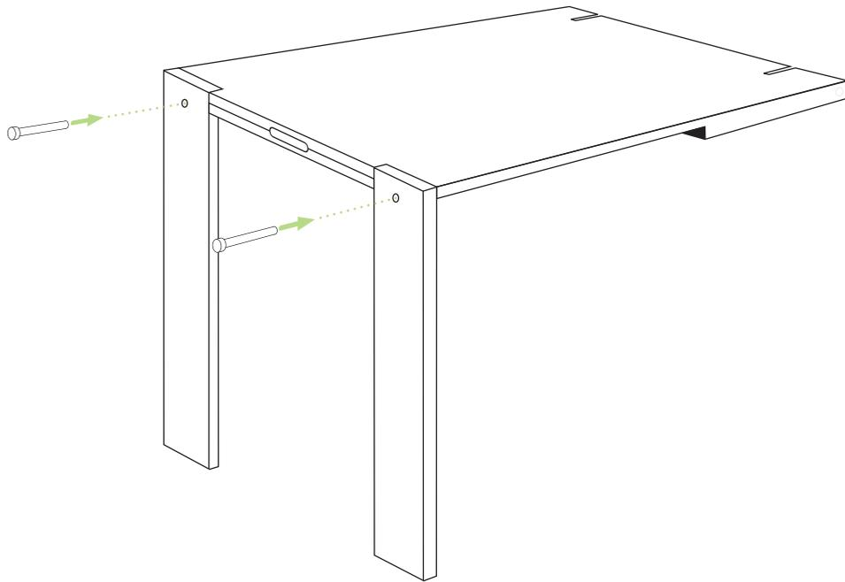
To lock the table legs insert the Bolts on either side of the table.
