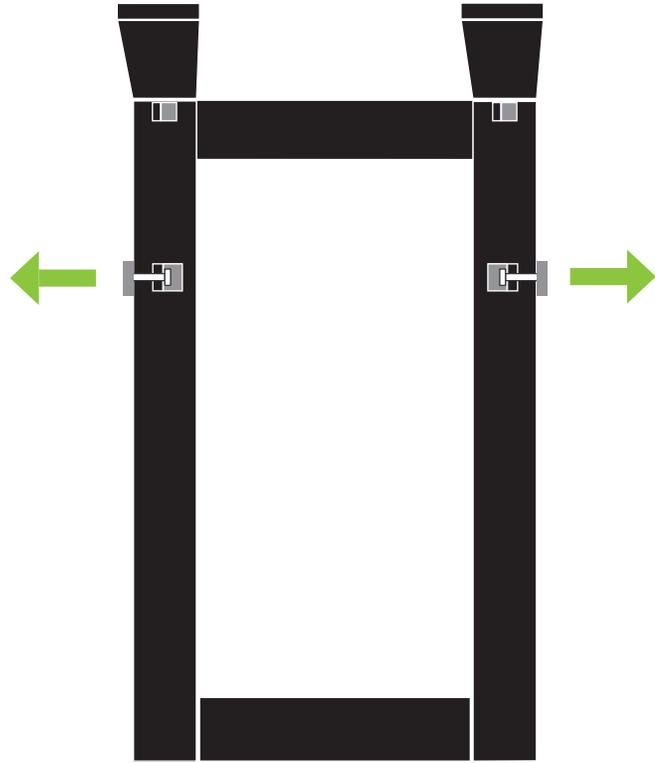
Push the **Upper Wall Mount Lock Bars** outwards into **the Upper Metal Lock**.
